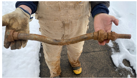
Removed Lead Gooseneck
